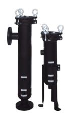
Pentair\* Industrial\* C44 Single Liquid Cartridge Housings give the versatility of choosing cartridges for the needed flow rates, chemical compatibility and particle retention. The C44 accommodates one element in 10", 20", 30" or 40" (254, 508, 762, 1,016 mm) lengths.
